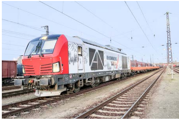
↳ Vectron Dual Mode Application: Traction for supply and disposal Drive: Electric (overhead line) and MTU diesel engine Top speed: 160 km/h Length: 19.98 m over buffers Traction power: 2,000 kW electric and diesel combined Weight: 90 tonnes
