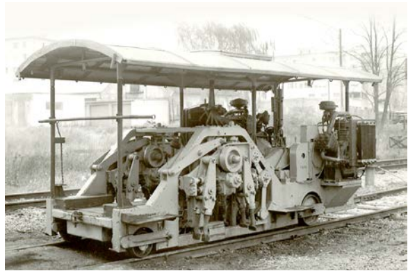
↳ This Matisa machine (1950) marked the beginning of the mechanised track construction era in Austria.
